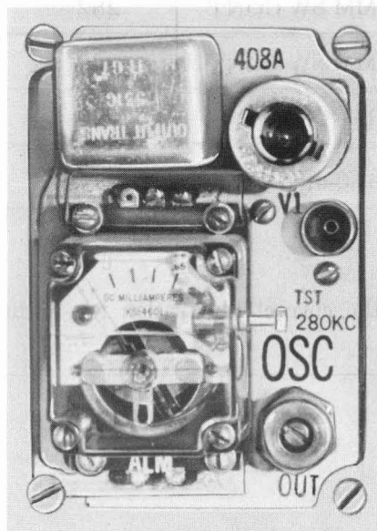
Fig. 1—Switching Signal Oscillator Unit (J68820B)
