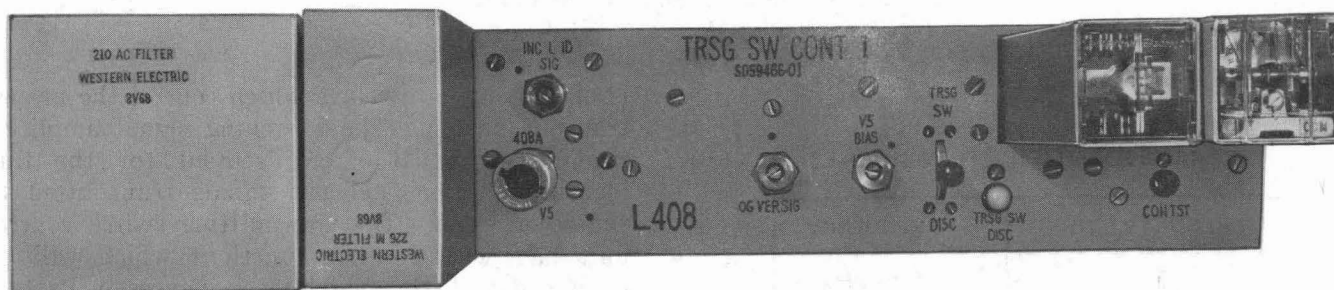
Fig. 6—Transmitting Switch Control Unit
