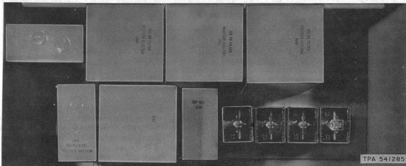
Fig. 9—Switching Signal Filter Unit
