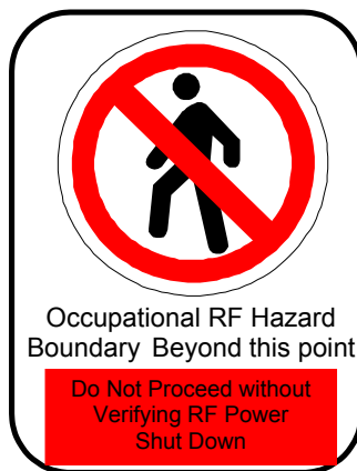
Example 2 – RF Hazard Sign
